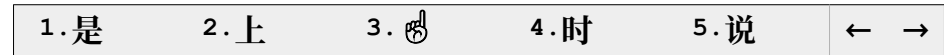
Menu display after typing the second letter h of the Pīnyīn sequence shìjiè.
